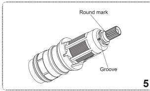
5. NOTE: Do not turn the cartridge when reinstalling it. If you turned it accidentally, you should adjust it and be sure that the round mark is correctly in line with the groove, or readjust as per the steps of verification and setting.
