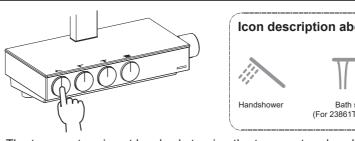
The temperature is set by slowly turning the temperature hand that limits temperature to 37°C. To get a higher temperature, p temperature handle counter-clockwise.
