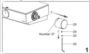
1. Before your action, make sure the number 37 on the temperature handle is upward vertically(It could not be turned counter-clockwise if not pushing the button). Remove the temperature handle(28).
